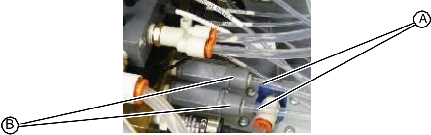
Figure 8.6: Prep station vacuum filters
