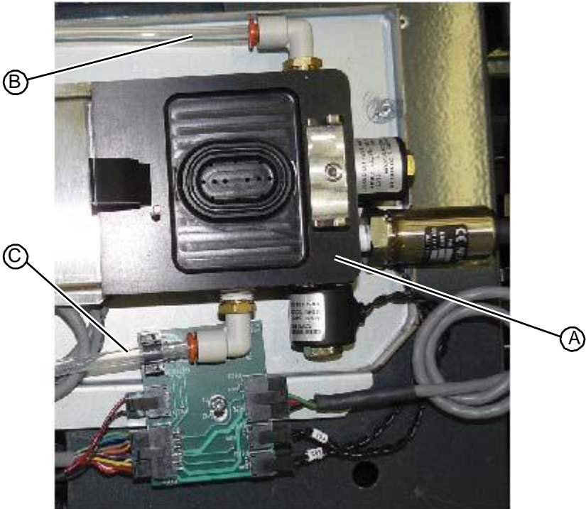
Figure 8.4: Prep station receiver plate assembly
