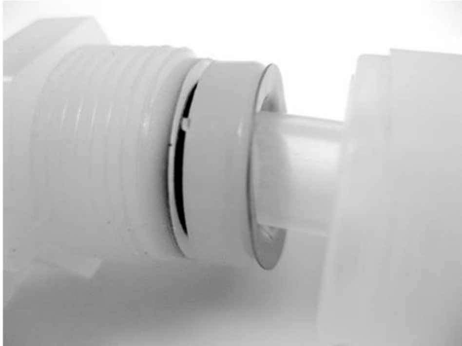
Figure 7.13: New Compression Fitting with Rings Properly Spaced
