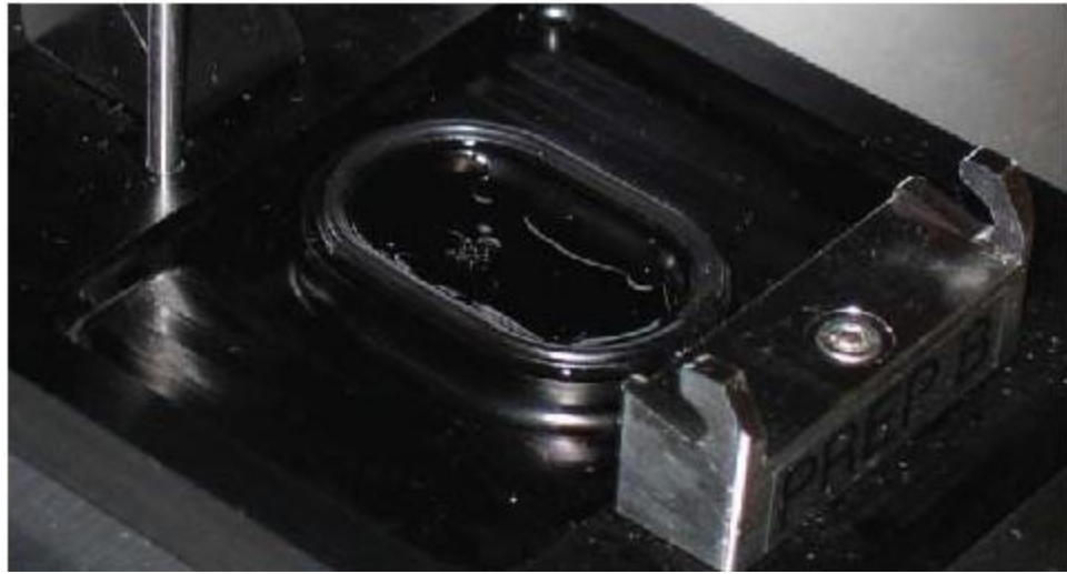
Figure 7.15: Example of bad flow at a prep station
