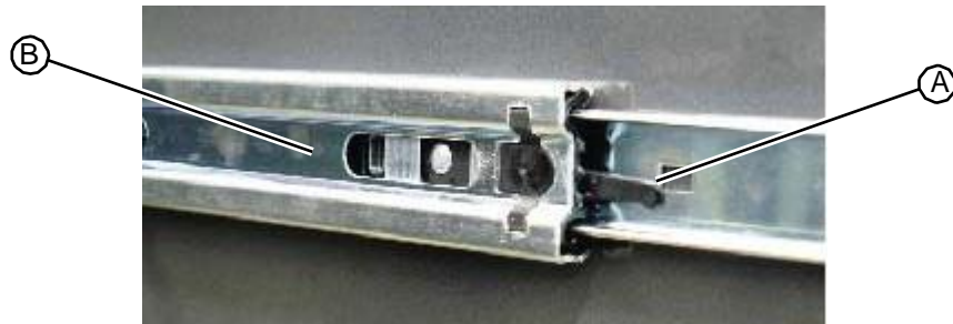
Figure 5.70: Track slide on the right side of the drawer
