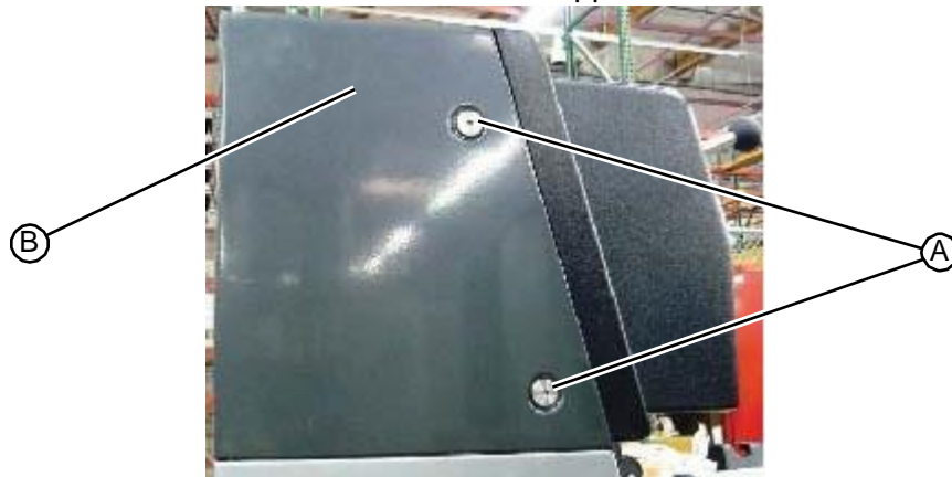
Figure 5.2: Fasteners located on the top of the upper hood
