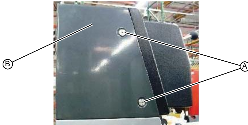
Figure 5.3: Fasteners located on the side of the upper hood
