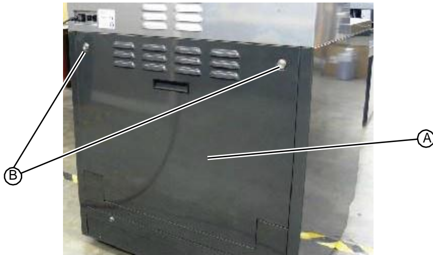
Figure 5.13: Fasteners that secure the rear access panel
