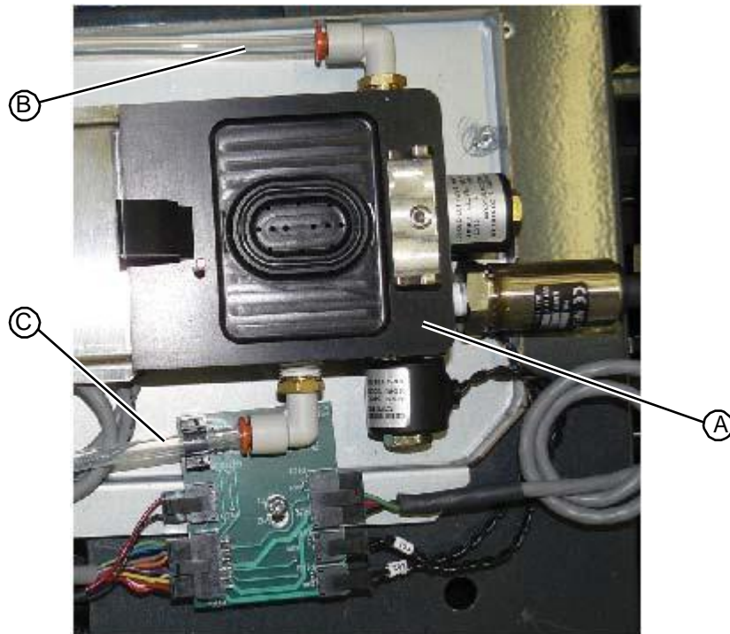
Figure 5.67: Tubing connected to the prep station manifold
