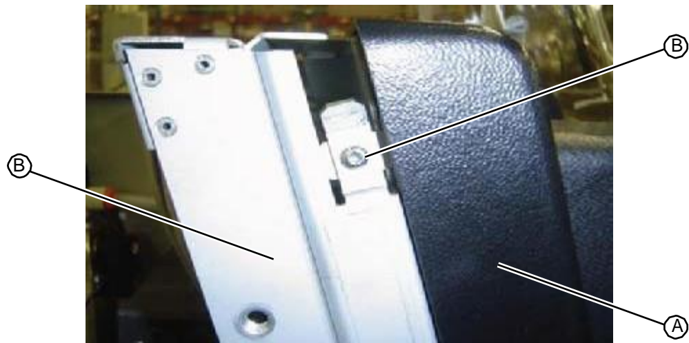
Figure 5.7: Drill side fascia fastener
