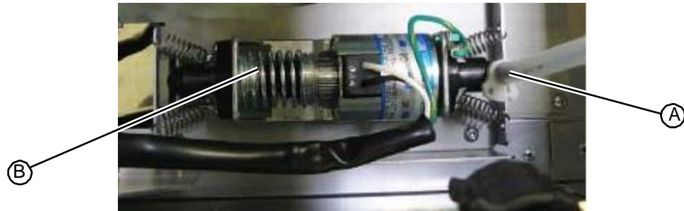
Figure 5.295: Tubing connected to the fluid pump that runs to the fluid distribution manifold
