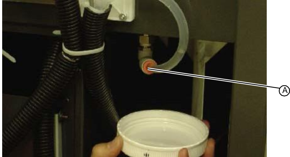
Figure 5.306: Disconnecting the line connected to the bottom of the liquid separator
