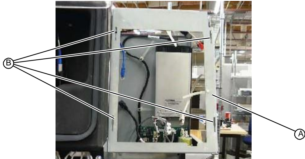
Figure 5.270: Touchscreen monitor mounting slots on the system frame
