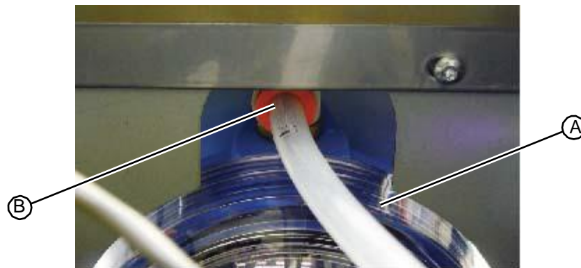
Figure 5.304: Vacuum cleanup wand tubing connection to liquid separator
