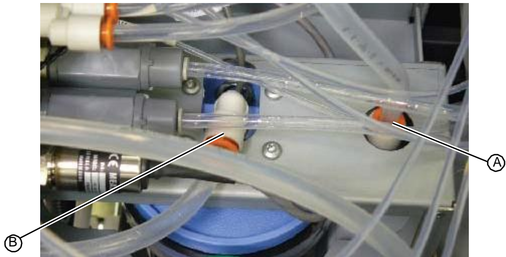
Figure 5.315: Tubing connected to the top of the liquid separator assembly
