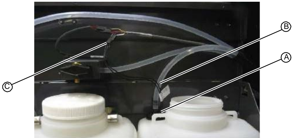
Figure 5.324: Level switch/siphon assembly tubing and cable connections
