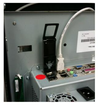
Plug the modem into the top left USB port (viewing the ports from the top).
