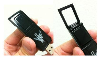
Modem antenna is folded for shipping. Unfold the antenna to improve reception
