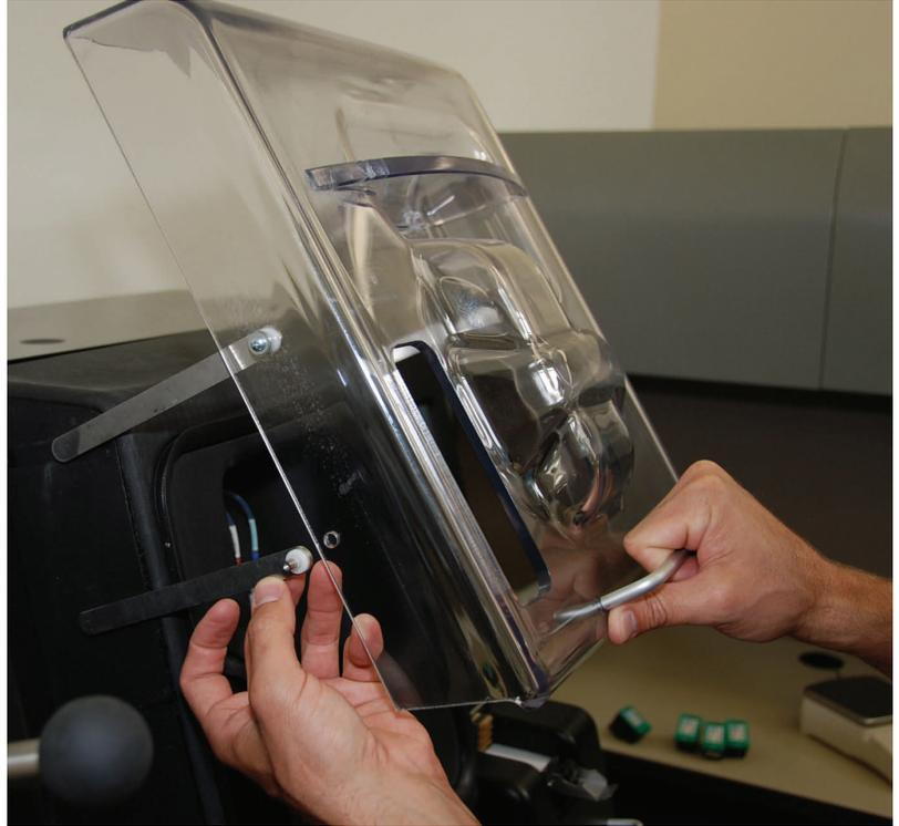
**B)** As before, Attach a bonded washer bushing with one of the four supplied screws, and secure it with a Phillips head screwdriver to the outside of each upper hinge arm. ***(Remember — do not over tighten the screws or they will snap off!)***
